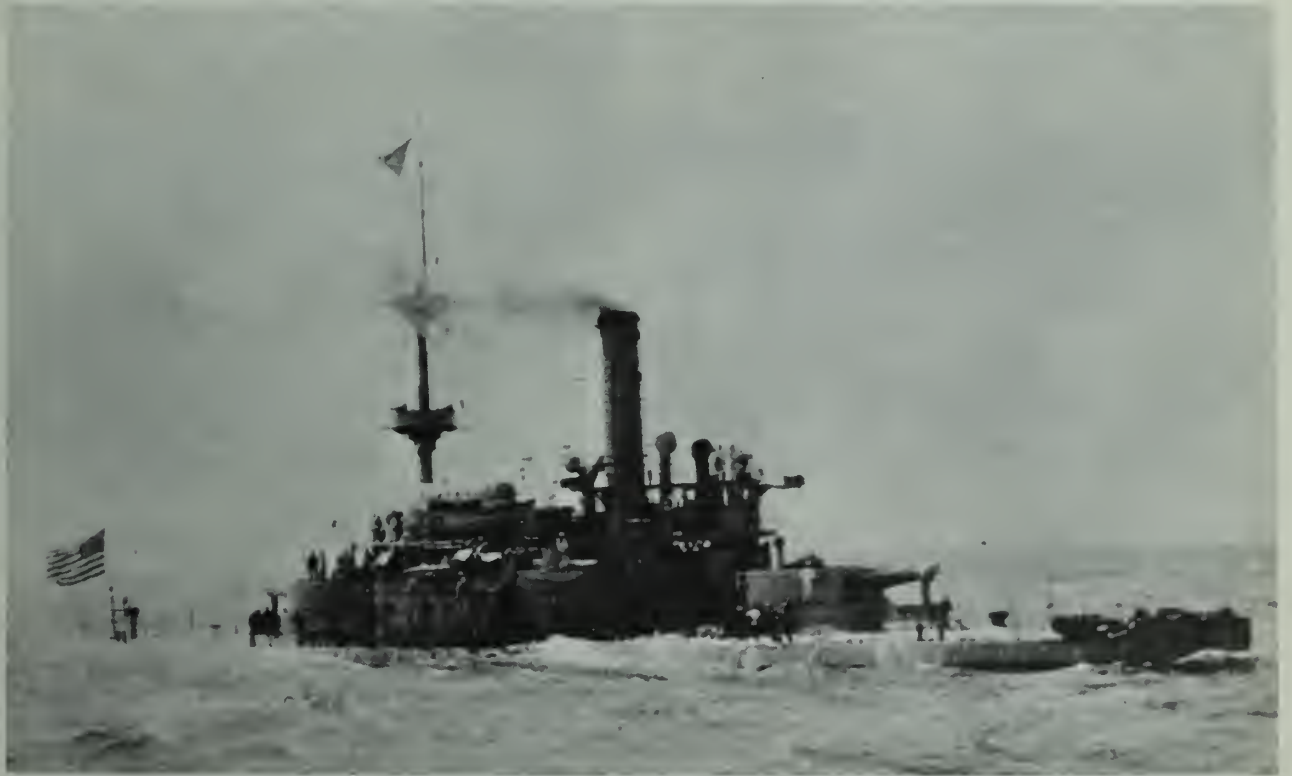
USS Monadnock enroute from San Francisco to Manila in 1898—Note the amount of water being taken over the main deck of the “new” monitor in a relatively slight sea.
